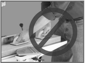
Figure 3. Never stand directly behind the workpiece!
